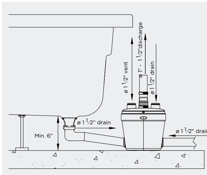
**AN EASY SOLUTION FOR A REMOTE LAUNDRY ROOM INSTALLATION OR FOR ANY GRAY WATER APPLICATION**
