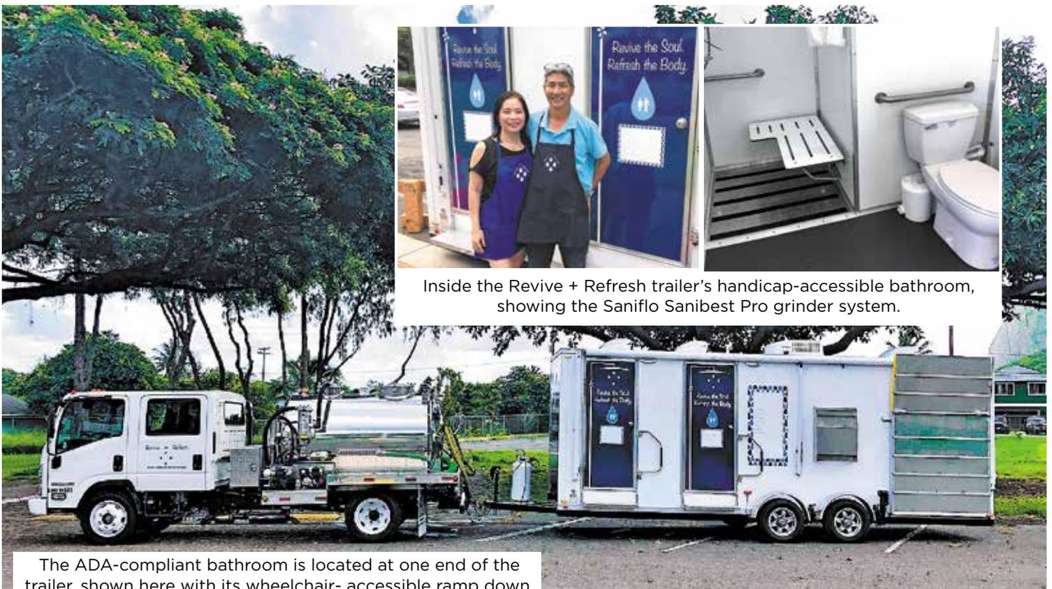
The ADA-compliant bathroom is located at one end of the trailer, shown here with its wheelchair-accessible ramp down.
