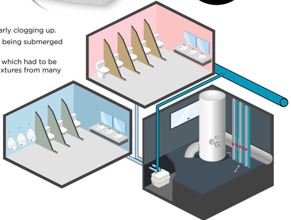
Sanicubic 2 grinder pump installed inside a pit where several bathrooms drained into the pump
