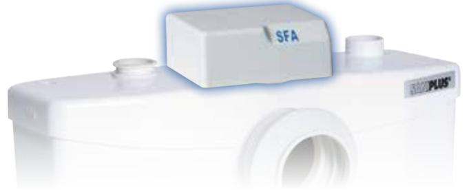
The Sanialarm has a level pressure switch that triggers an alarm fixed on the top of the unit if the volume of water exceeds the maximum allowed level. The alarm emits a continuous 80 dB warning sound until it is switched off or the problem is rectified. The Sanialarm is battery operated and can be installed on most Saniflo macerating units and drain water pumps.
