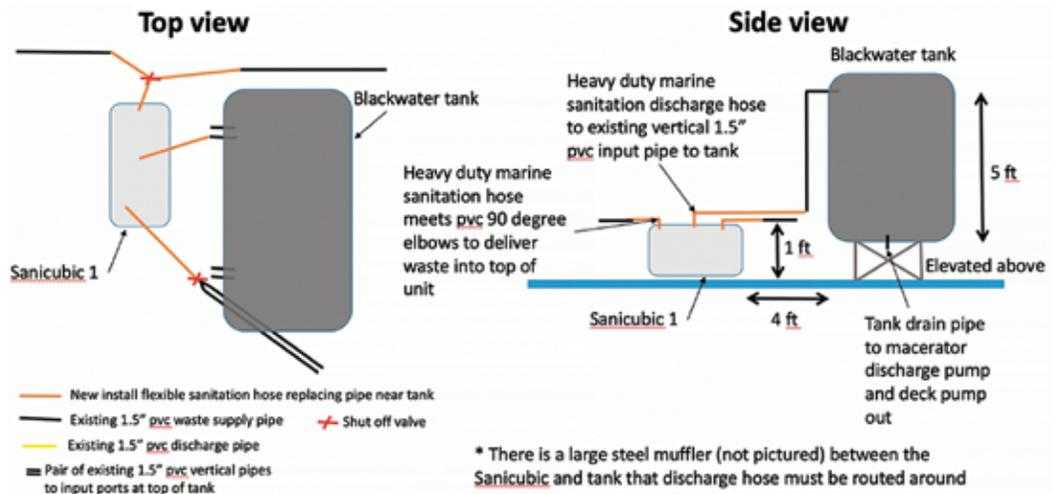
\* There is a large steel muffler (not pictured) between the Sanicubic and tank that discharge hose must be routed around
