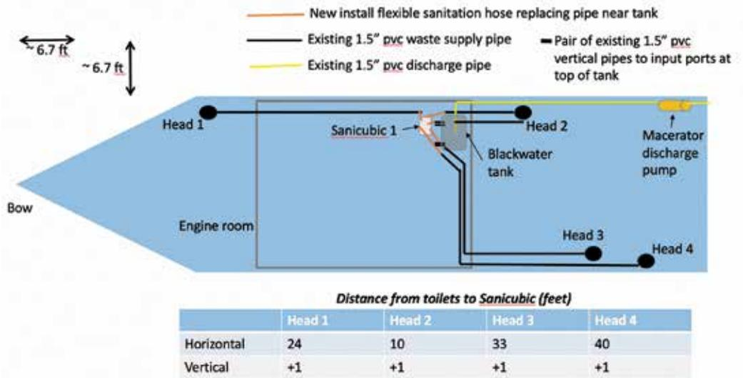
Sanicubic ~ 5 ft below existing input port at top of black water tank
